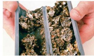
(a) Clogging a pipe
