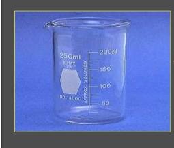
Hold and/or heat solids or liquids that will not release gases when reacted, or are unlikely to splatter if stirred.
