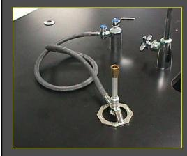
used for the heating of <u>nonflammable</u> liquids and solids.
