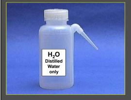
has a tip that delivers a stream of water to a specific area when squeezed.
