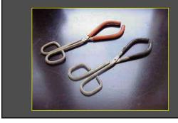
used to hold and move beakers containing hot liquids.
